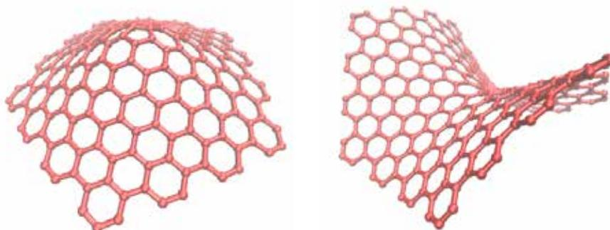
Distorted geometry of a graphene sheet containing a single pentagon (left) and heptagon (right), which can be considered as disclinations with positive and negative disclinations.
