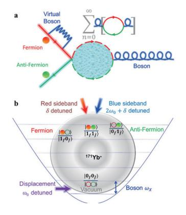
Figure 1 Fermion-antifermion scattering process and its mapping to a 171Yb+ ion system. (a) Diagram of the interactions between a fermion, an antifermion, and bosons. (b) Diagram of the encoding and operation to implement the interaction Hamiltonian with a 171Yb+ trapped ion.
