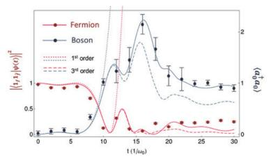
Figure 2 Trapped-ion simulation results of quantum field theories. Fermion and antifermion annihilation process in the strong coupling, where both the self-interaction and pair production processes strongly influence the dynamics.
